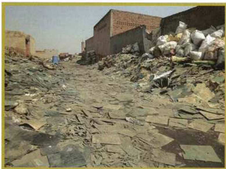
The town of Mandoli, about two hours from Delhi, is a center for the informal acid-stripping of copper from circuitboards denuded of their precious-metals-bearing components.
