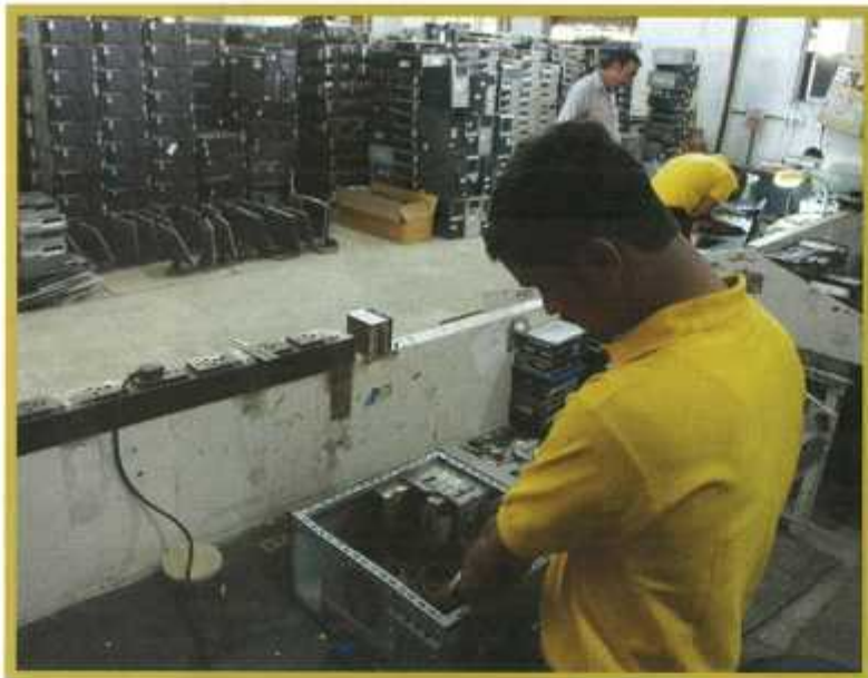
Eco Recycling—or Ecoreco—is a licensed dismantler and recycler with a substantial reuse and refurbishment business. Here, a company technician refurbishes a desktop PC (above left) to sell in India's thriving reuse market. In another part of the facility, a worker feeds PC cases into a shredder (above right).
